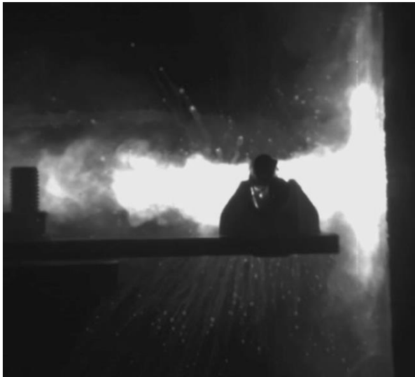
Figure 2.2-1 – 3 kV DC electrical arc impacting structure thermal runaway
